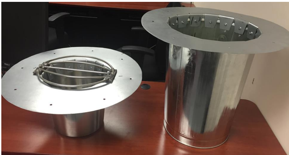
Figure 1. The two buckets comprising the “bucket in a bucket” collection device. Left: smaller, inner bucket serving as collection basin for drooled saliva. A grate, that can be removed when deposited saliva is being collected, covers opening. Right: larger, outer bucket housing ice and scent wicks. Bolts and acorn nuts hold buckets together, while also securing device to wooden housing. (Sgambelluri, 2017)
